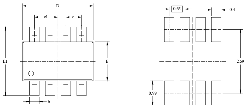
RECOMMENDED LAND PATTERN (Unit: mm)
